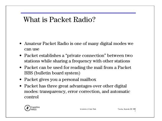
The operation of a packet station is transparent to the end user; connect to the other station, type in your message, and it is sent automatically. The Terminal Node Controller (TNC) automatically divides the message into packets, keys the transmitter, and then sends the packets.
