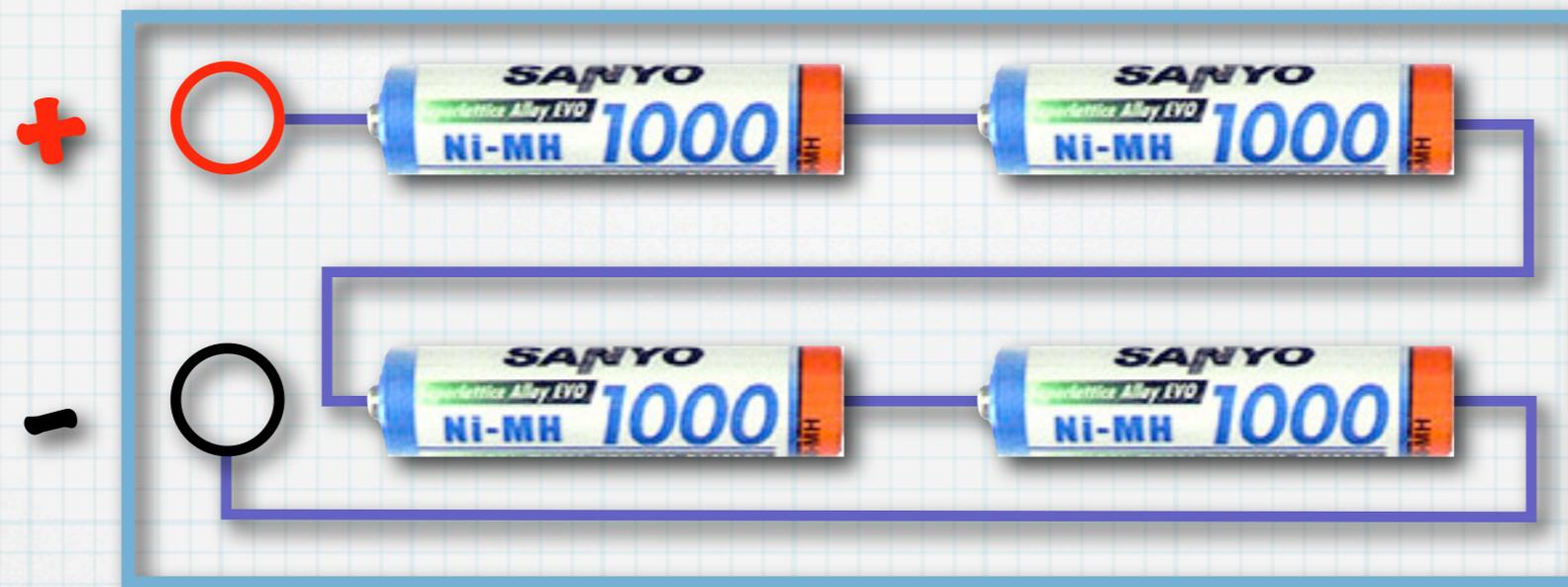
Made up of multiple cells in series
