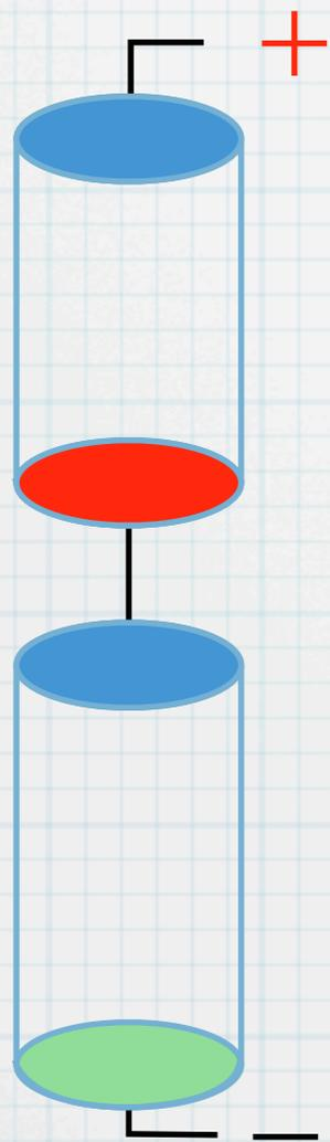
The upper cell has less capacity than the lower one
