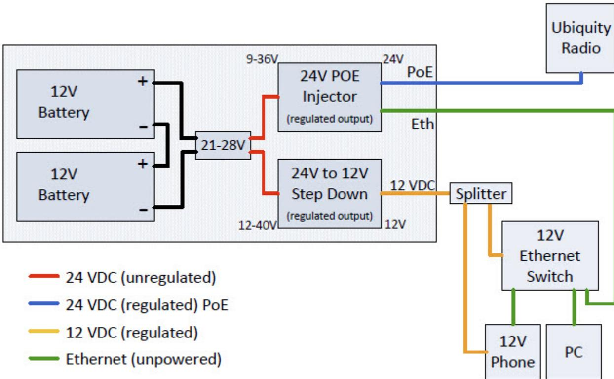
**Example power configuration for powering Ubiquiti devices from batteries.**
