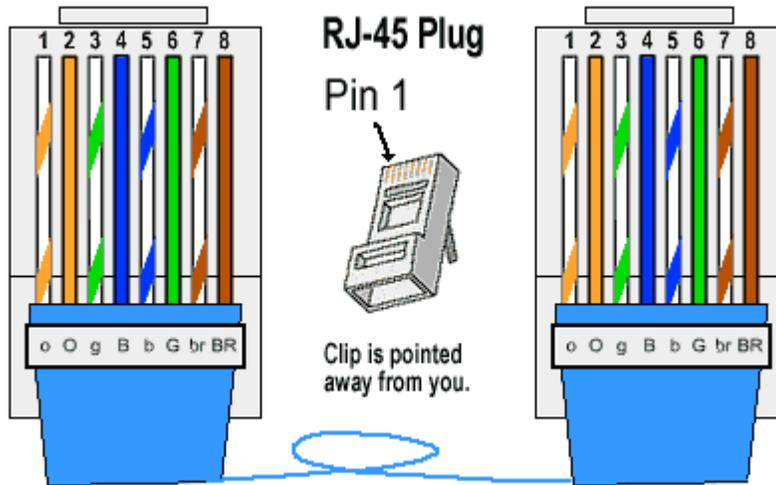
2. **Crossover Cable.** These cables directly connect one computer to another computer (or device) without going through a router, switch or hub.
